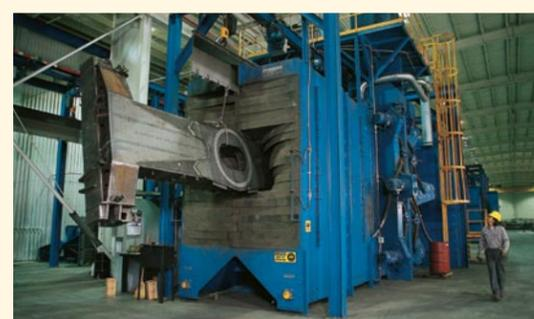
A 12-WHEEL BLAST CABINET and 48-foot paint booth exemplify the super-sized equipment at O'Neal's weldment operations.
